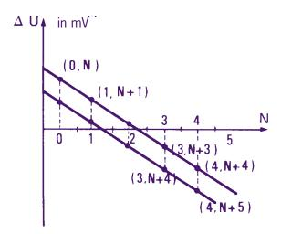
The neutral point is determined by interpolation between the intersection of the two voltage drop curves with the horizontal abscissa.
