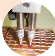
\*CL-Profiler, the solution for profiling slip ring assemblies and commutators
