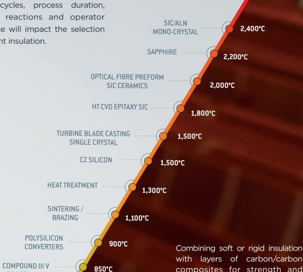
TYPICAL RUNNING TEMPERATURE - INDICATIVE T° VALUES WITH USUAL PRESSURE ON INDUSTRIAL PROCESS (10-2)
